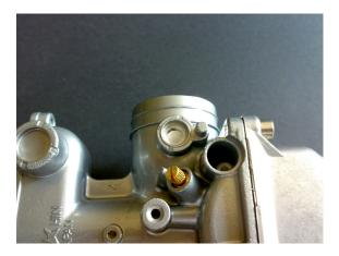
Pop the tee back into the hole to firmly seat the O-Ring in place.
