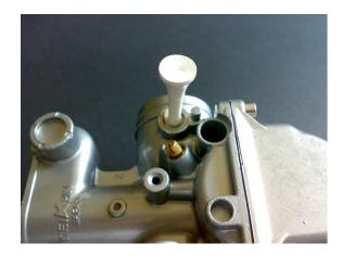
Remove the tee and use the watch pin remover to poke the rest of the O-Ring into the groove.
