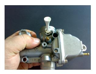
Use the watch pin remover to poke the lip of the O-Ring into the groove.
