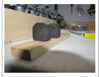
2.20 Repeat for remaining carbs and then check floats, and valves are working the same. I had to replace a Keyster valve as it compressed more easily than the others.
