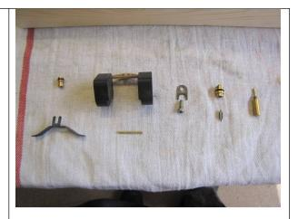
1.6 Remove the needle jet using a bamboo meat skewer. If the needle jet is stuck and won't move, try pushing it down gently from inside the carb throat, by opening the needle slide and using the blunt end of the bamboo stick.
